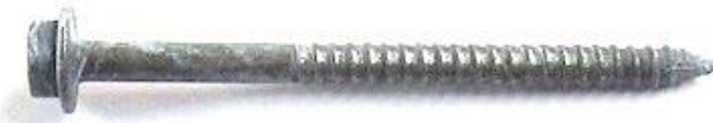
Sample FM-X5 -3DG Grey/ Opaque n. 5 End of the test after washing for salts removal
