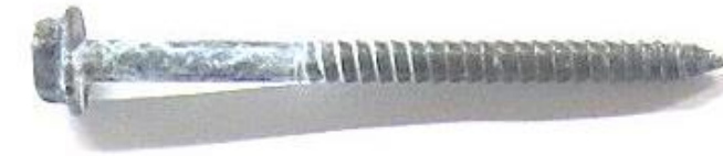
Sample FM-X5 -3DG Grey/ Opaque n. 4 End of the test after washing for salts removal
