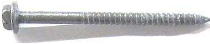
Sample FM-X5 -3DG Grey/ Opaque n. 2 End of the test after washing for salts removal
